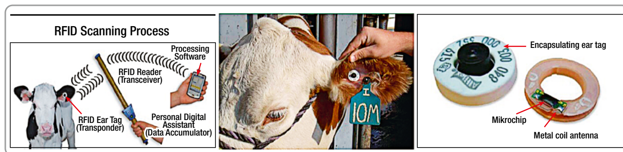
Figure 3. A sample of RFID tags and their function
