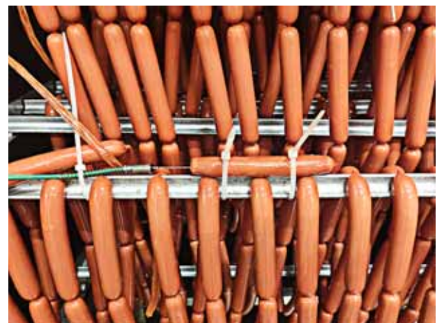
Figure 5. Probe placed in the thermal center of the product on a cart
