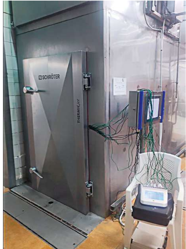
Figure 1. Schroter chamber with thermocouple probes observed from the side in the thermal processing room.
