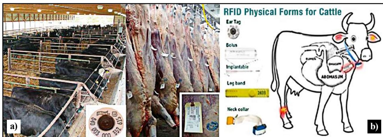
Figure 5. a) Application of RFID in animals from birth and throughout the breeding period until arrival at the slaughterhouse and sending their meat to stores; b) Different locations for the installation and use of RFID tags in a live animal
